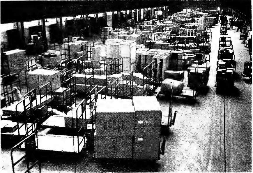
Fig. 3—Freight house of the Chicago, Burlington & Quincy Railroad at Morton Park, Ill., showing in-floor towing conveyor in operation.
